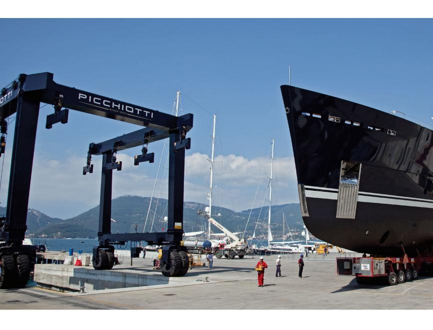
ABOVE: The Picchiotti shipyard in La Spezia has a spectacular location and an 820-ton travel lift that allows the yard to launch such large vessels as *Galileo G*
